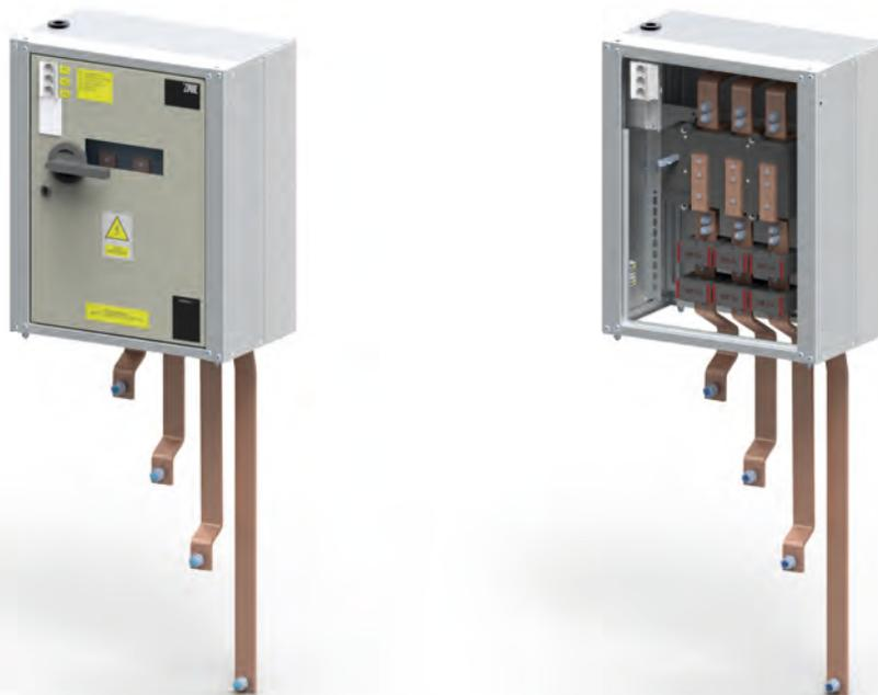
In the incoming module, an INP 1000–2000 switch disconnector or other manufacturer's switch disconnector (after consultation) or compact circuit breaker with rated current (630 – 1600 A) can be installed. The circuit breaker or switch disconnector can be equipped with a motor-drive mechanism. It is also possible to install ammeters, voltmeters or a network analyser.
